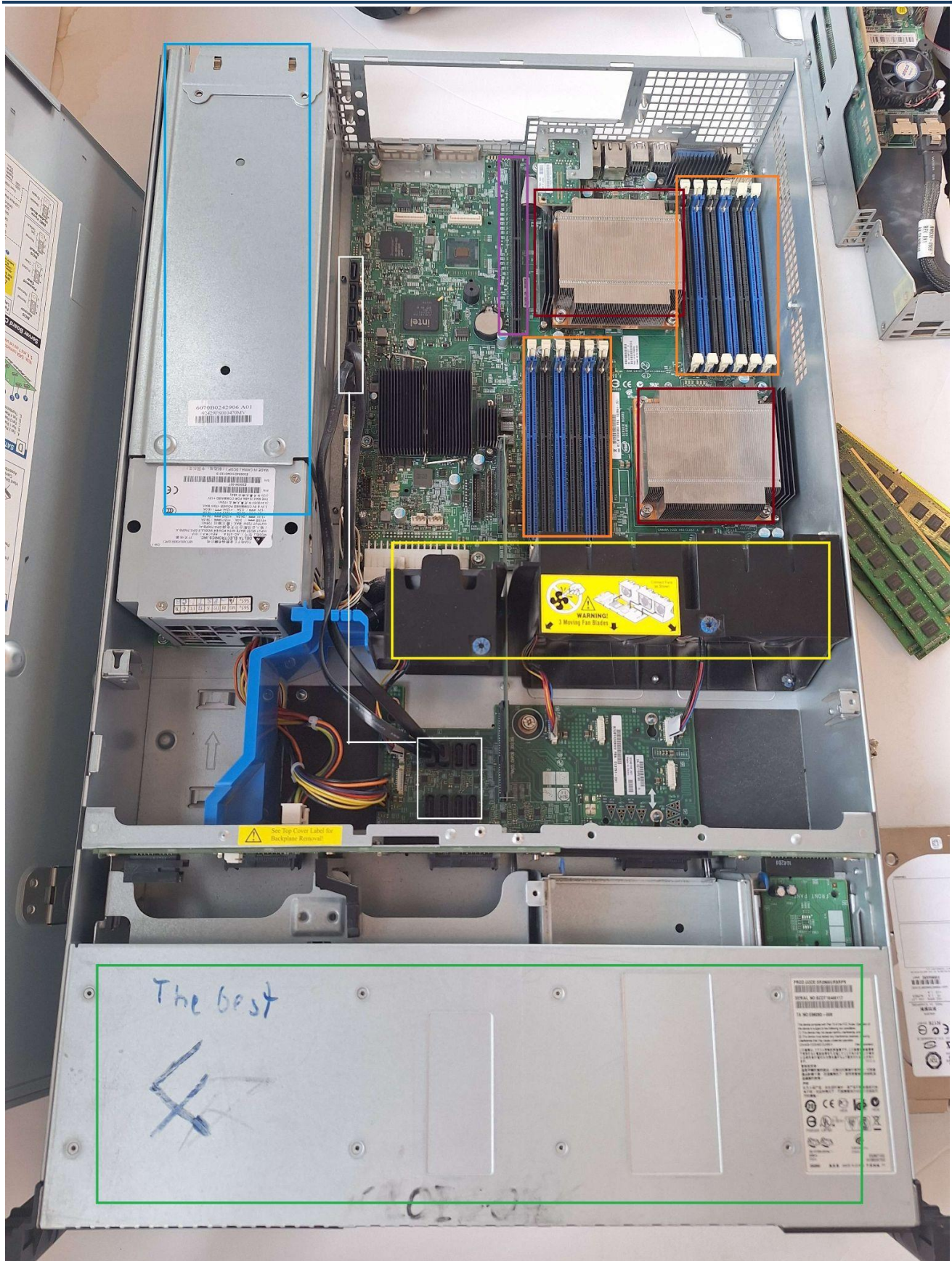
Internal layout — motherboard, CPUs, RAM, and storage
