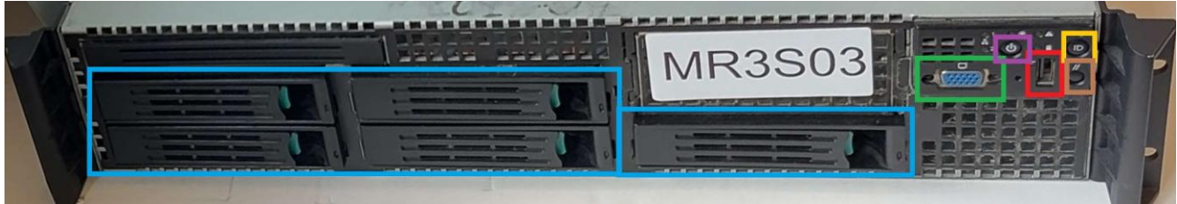
Front panel — drive bays and control buttons
